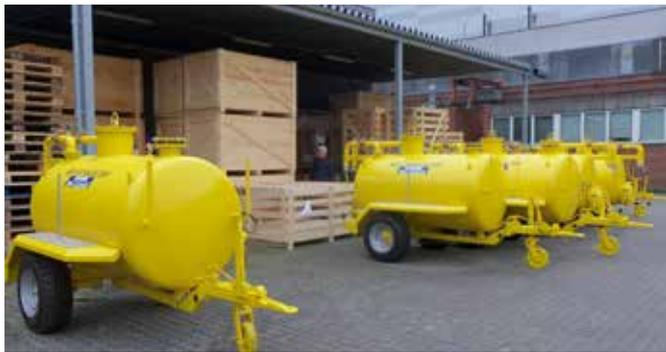
The RO-TANKER is fitted with large diameter wheels for off-road towing and a large diameter access hatch at the rear.
