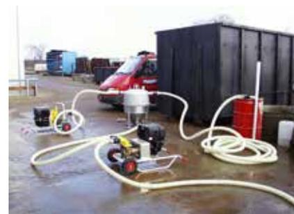
The RO-VAC MINI pump can be supplied to pump the recovered oil from the storage hopper to further storage or tanker. Indeed, the pump can be used as a stand-alone, diesel driven unit for use on other duties.
