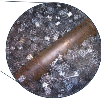
Column filled with aluminium packing rigs
